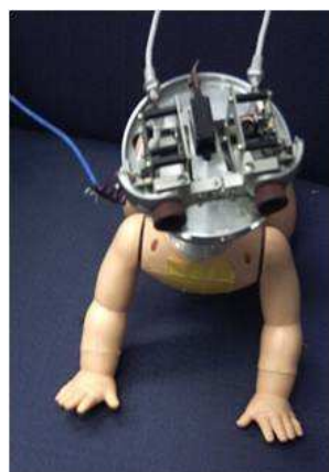
Figure 4. Mark 2 Robot Baby, has 2 USB AV webcams mounted with additional eye convergence motor.
